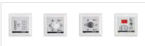
Programme switches for selection of automatic door operating modes. Up to 5 different operating modes can be set: Off, Night, Shop closing, Automatic and Permanently open.
